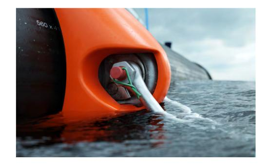
The insert is fitted to the welded mooring lug on the mooring bracket, and acts as a replaceable lining that can be worn out. The mooring lug insert can be retrofitted at sea, or supplied pre-fitted to floating collars during production. This fitting means that aquaculture operators avoid the need to replace the full mooring bracket when wear and tear exceeds the set limits.
