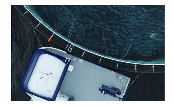
Large Boat Mooring ensures safe and gentle mooring of wellboats and larger vessels while extending the lifespan of the floating collar and reducing stress on the mooring brackets. With easy installation and efficient load distribution, this solution enhances operational reliability and minimizes unexpected maintenance needs.
