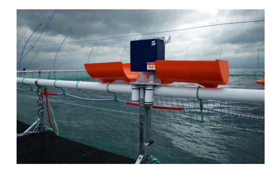
ScaleAQ's electrical cabinet module protects electrical cabinets on both our own pens and those from other suppliers. The cabinet provides protection from the elements, and ensures that the cabinet is securely fitted to the pen. The module is compatible with ScaleAQ's universal bracket for extra equipment.
