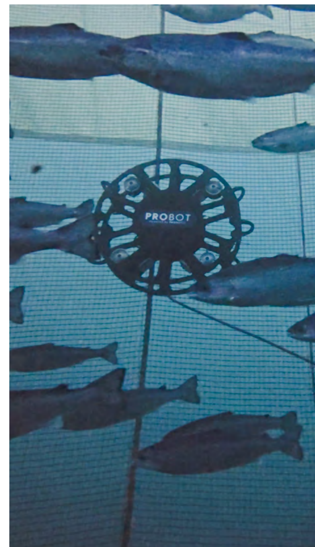
PROBOT is an autonomous underwater robot. Efficient, environmentally friendly, and autonomous cleaning and inspection of nets – designed to ensure optimal fish health and extend net lifespan.
